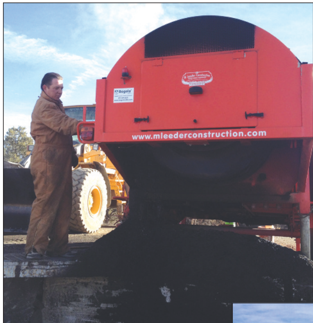
Setting the Bagela on an elevated pad allows it to dump the recycled product directly into asphalt trucks and trailers below.
