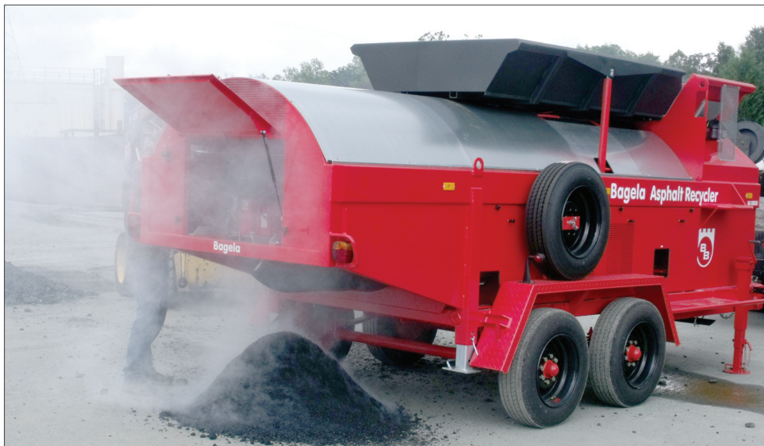
Bagela manufactures three different sizes of asphalt recyclers: BA4000 (4-ton [3.6 t]), BA7000 (7-ton [6.4 t]) and BA10000 (10-ton [9 t]).
