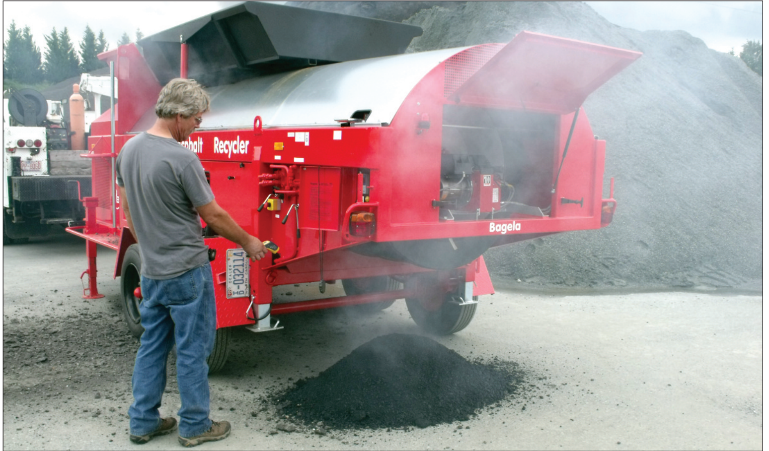
The Bagela asphalt recycler line is designed to supply hot asphalt on demand using existing RAP, chunks, millings or leftover plant mix.
